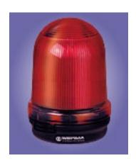
The beacon lamp is comprised of four rows of LED diodes in appropriate colour according to order. It is all-plastic with double insulation and IP 65 protection. The fixing points are at the bottom of the lamp as well as the rubber cable bushing. The beacon has no protection against cable pulling; therefore the cable must be mounted firmly all the way to the bushing. The picture below shows the recommended lamp position. This position is obligatory for outdoor use.
