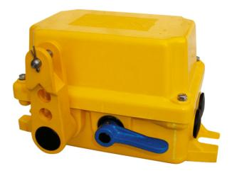
Cable emergency switches are used for quick switching off conveyor belts or other large machines and equipment by pulling the cable connected with a switch. Cable emergency switches serve as a protection e.g. at a fall on the conveyer, trapping by a machine or towing by the cable etc.
